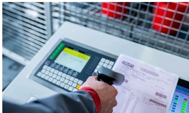
Scanning of the product code before the filling process
