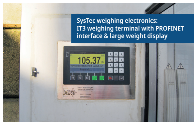
Belt scale in soil cleaning plant in Alkmaar (photo above) and IT3 weighing terminal (photo below)
